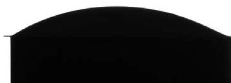
Figure S3. Water droplet on tablet of functionalised silica nanoparticle (triethoxymethylsilane : trimethoxy(octyl)silane = 160 \mu\text{L} : 40 \mu\text{L} ). The total silane to nanoparticle ratio was kept constant at 200 \mu\text{L} \cdot \text{g}^{-1} .
