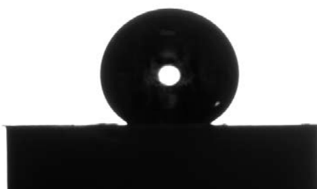
Figure S5. Water droplet on tablet of functionalised silica nanoparticle (triethoxymethylsilane : trimethoxy(octyl)silane = 120 \mu\text{L} : 80 \mu\text{L} ). The total silane to nanoparticle ratio was kept constant at 200 \mu\text{L} \cdot \text{g}^{-1} .
