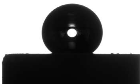
Figure S6. Water droplet on tablet of functionalised silica nanoparticle (triethoxymethylsilane : trimethoxy(octyl)silane = 100 \mu\text{L} : 100 \mu\text{L} ). The total silane to nanoparticle ratio was kept constant at 200 \mu\text{L} \cdot \text{g}^{-1} .
