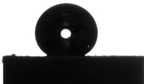
Figure S4. Water droplet on tablet of functionalised silica nanoparticle (triethoxymethylsilane : trimethoxy(octyl)silane = 140 \mu\text{L} : 60 \mu\text{L} ). The total silane to nanoparticle ratio was kept constant at 200 \mu\text{L} \cdot \text{g}^{-1} .
