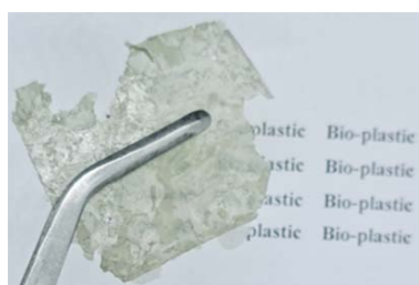
Fig. S11 The digital image of the COE-11 sheet prepared by hot-pressing (180 °C, 10 MPa, 5 min).
